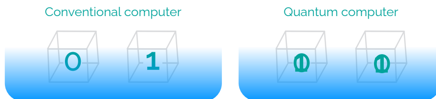
Figure 5: A bit of a conventional computer can only ever assume the value 0 or 1. In a quantum computer bit (Qubit), on the other hand, both states are possible at the same time. Qubits can therefore be used to perform several calculations simultaneously.
